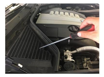
Lever out expanding rivet. Release locks in direction of arrow. Feed out fresh-air duct (1) and remove
