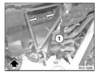
Open clamps. Release lock (1) in direction of arrow. Remove cover (2).
